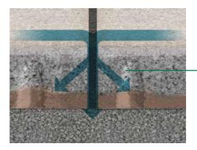
The surface infiltration for the GDM.KLIMASTEIN serves as a practical flood protection, it relieves the drainage systems and sewage treatment plants and recharges the groundwater. The system with aBG acts like a treatment facility for rainwater, ensuring reliable groundwater protection. Thanks to its innovative three-layer structure, the GDM.KLIMASTEIN achieves significantly higher evaporation rates than conventional systems.
